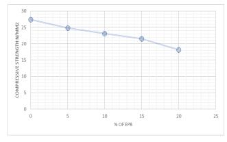
From the above analysis, for no replacement mix, 0% EPB, the strength obtained as 27.45 N/mm², and then it was reduced for every addition of EPB. 24.8 N/mm² was obtained for 5% replacement, for the 10% replacement it was noted that 23.1 N/mm², 21.5 N/mm² is the tested value of 15% replacement and finally for the 20% replacement the obtained compressive strength is 18.2 N/mm²
